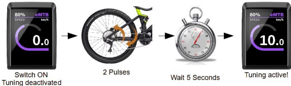
After the 5 seconds, the speedometer shows **10 km/h** for a few seconds to indicate the activated Tuning.
