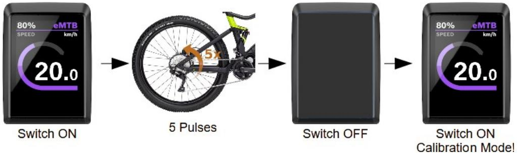
The **Calibration Mode** is now active and a **permanent** speed of about 20 km/h is displayed. By moving the magnet in front of the sensor you can now set the displayed speed to 20 km/h:
