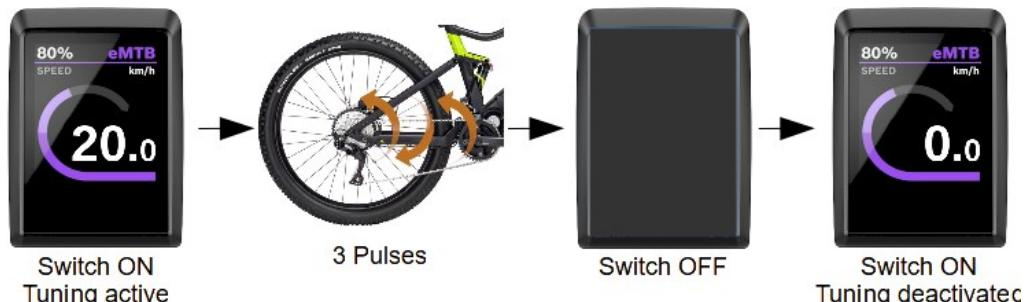
After switching on, the speedometer shows **0 km/h** to indicate that the Tuning has been deactivated.
