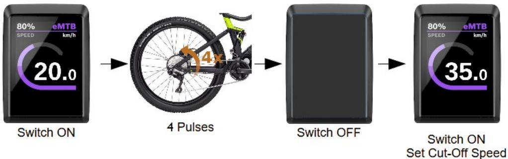
The mode for setting the maximum support speed is now active and the speedometer shows the current setting (e.g. 35 km/h). By moving the magnet past the sensor, you can now go through all the setting options:
