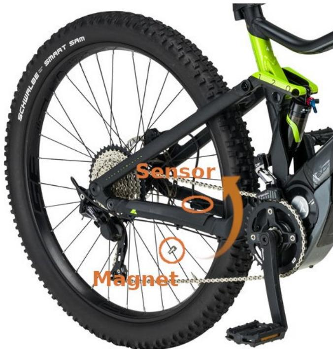
The magnet is attached to the spokes of the rear wheel. The speed sensor is attached to the frame so that the magnet passes it every time the wheel turns. Ideally, you lower the bike slightly to the left over the bike stand, so you can easily move the rear wheel by hand.
