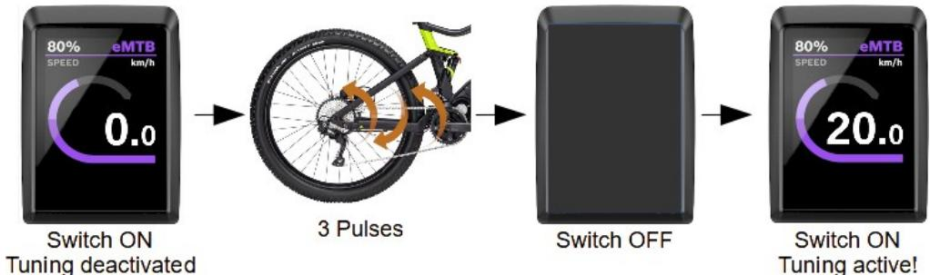
To indicate the Tuning is operational, the speedometer shows **20 km/h** for a few seconds.
